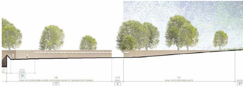
Figure 24. Elevation specifies a 12 foot gap where a trail passes between the upper and lower sections of Memorial Wall.
